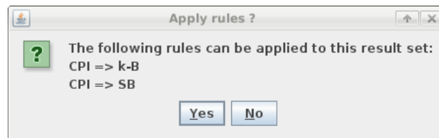
Fig. 3. Charlie asks the user for applying a rule. As one can see, Charlie handles each property separately. Thus, there is a rule for “k-bounded”, and there is a rule for “structurally bounded” as well, although the property “structurally bounded” implies the property ‘k-bounded’.
